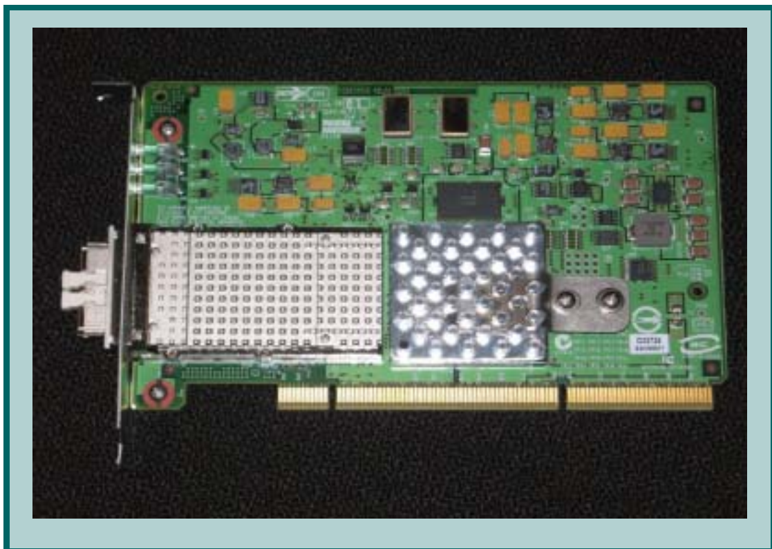
Figure 1 AD385A PCI-X 10 Gigabit Ethernet Card
